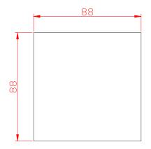
The AIM-T300 insulation monitoring device adopts embedded installation, and the above diagram is the hole dimensional drawing of the insulation monitoring device.
